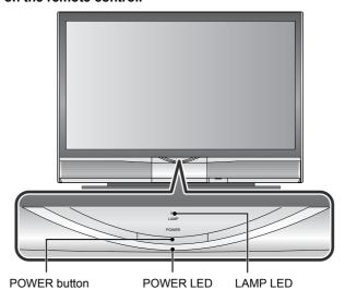
When the POWER button is pressed, the POWER LED lights up and the LAMP LED indicator blinks in orange for approximately 1 minute at approximately every 2 seconds.
